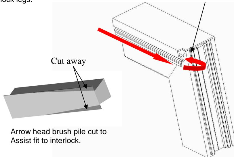
6. Cut gasket Articles 219350 & 219360 4mm longer than the lower sash they are fitted to (as per REHAU Manufacturing Recommendations). This will help reduce draughts that may circulate around the bottom sash.
