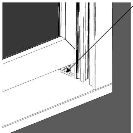
4. Adding a further 3mm length to the internal interlock (1.5mm per side), helps reduce draughts plus with the bonus of reducing side to side motion keeping the sash in a more central position between brush piles.
