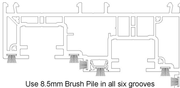
2. Fitting the Aluminium security bar, (Art. 219290) to the Sill not only adds improved security but also improved weather performance by means of its additional brush pile against the front bottom sash.
