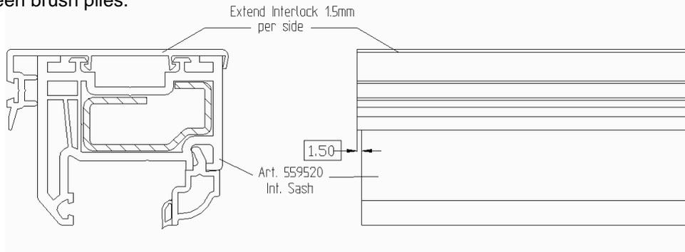
5. We leave at least 20mm of brush pile either side of the interlocks (as per REHAU manufacturing recommendations) which can be tucked around the back of the interlock. The brush pile ends may need to be cut to a slight arrow head in order to aid the location between the interlock legs.
